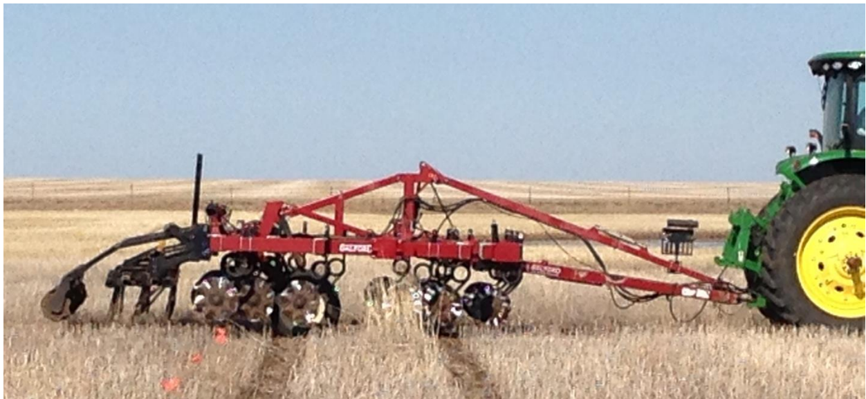
Figure 2. Salford vertical tillage implement used in demonstration
