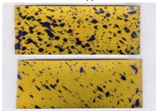
Dual Nozzles & 18 inches above canopy "Sub-optimal" Fusarium application
